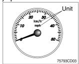
① The speedometer displays the speed of machine in mph and km/h.
