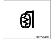
① This lamp comes ON when mirror defrost switch is pressed.
